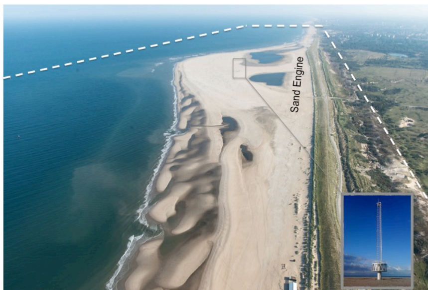
Fig. 1. Aerial photo of the proposed ICON.NL location. The Sand Engine is the region of anomalously wide beach while the adjacent Kijkduin beach segment is the straight beach to the north. The tall tower visible in the centre of the Sand Engine is the location of several of the proposed remote sensing instruments. Note the large spatial variation in waves and beaches in the location of interest.
