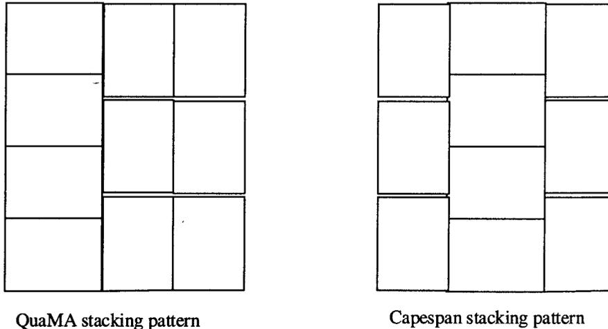
figure 3 Stacking patterns used in the experiments for the two different boxes.
