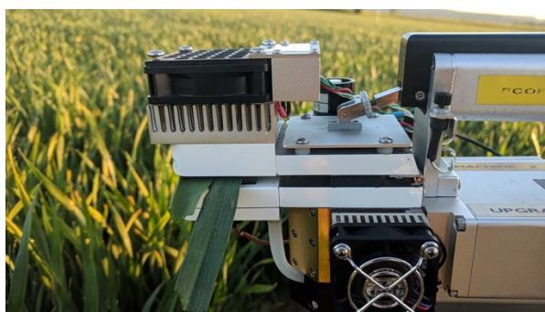
Figure 2.1 LI-6400XT used in the CloudRoots campaign to measure the leaf gas exchange
