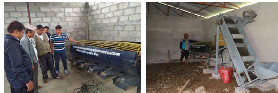
Photo 5.8 Potato grading machine start up and below Potato elevator machine for facilitating grading of potato (Source DACF)
