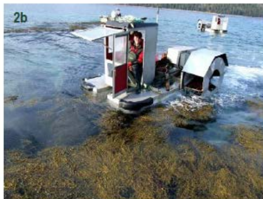
Figure 2: Harvesting methods for a) Lamniaria hyperborea , the seaweed trawl and for b) Ascophyllum nodosum the paddlewheel cutter. Photos: a) FMC Biopolymer AS, b) Sander Andersen (5)
