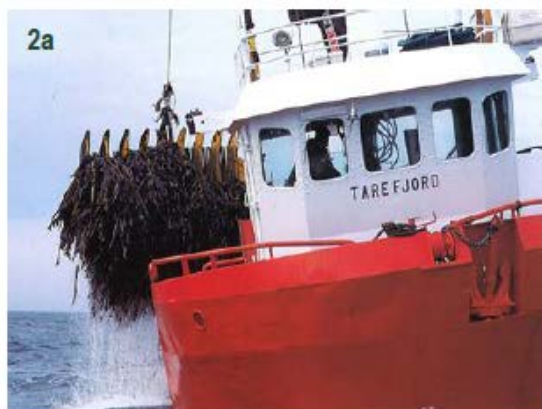
Figure 2: Harvesting methods for a) Lamniaria hyperborea , the seaweed trawl and for b) Ascophyllum nodosum the paddlewheel cutter. Photos: a) FMC Biopolymer AS, b) Sander Andersen (5)
