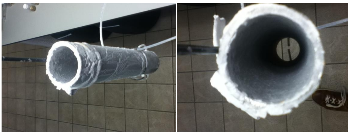
Figure 19: Thin layer of struvite or magnesium oxide on a stainless steel pipe
