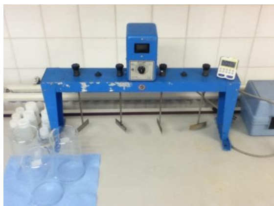
Figure 8: Jar test setup, 4 stirrers rotating at equal speed
