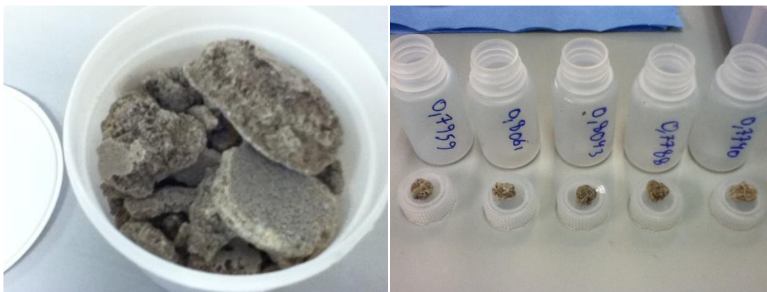
Figure 6: Left: struvite from a WWTP pipe, right: struvite cut into uniform sizes for testing
