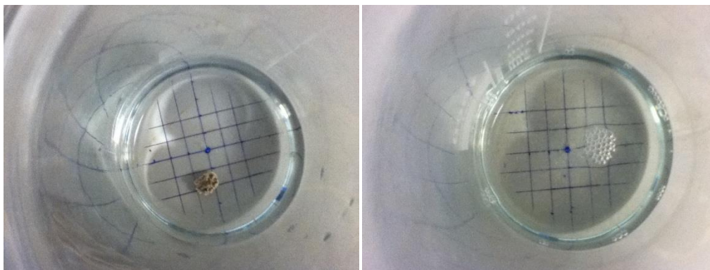
Figure 14: Start (left) to finish (right) of 0.8 g MAP in 1M HCl ~45min. mixing
