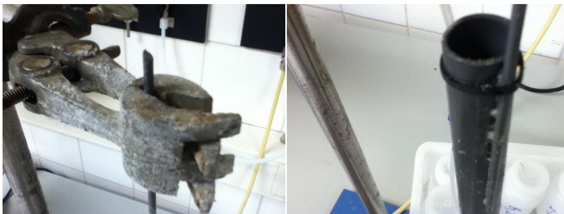
Figure 17: Struvite on the clamp and on the outside of the pump
