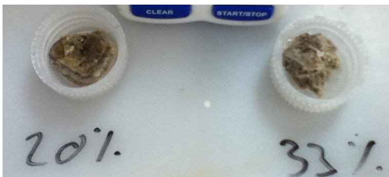
Figure 22: Start of test ~3g of MAP reacts with 5M and 8.25M caustic soda
