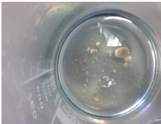
Figure 16: Soft struvite in a 8.25M NaOH solution after 120 minutes of mixing
