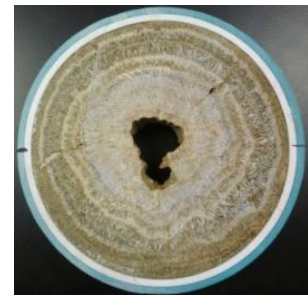
Figure 4: Struvite clogged pipe [47]
