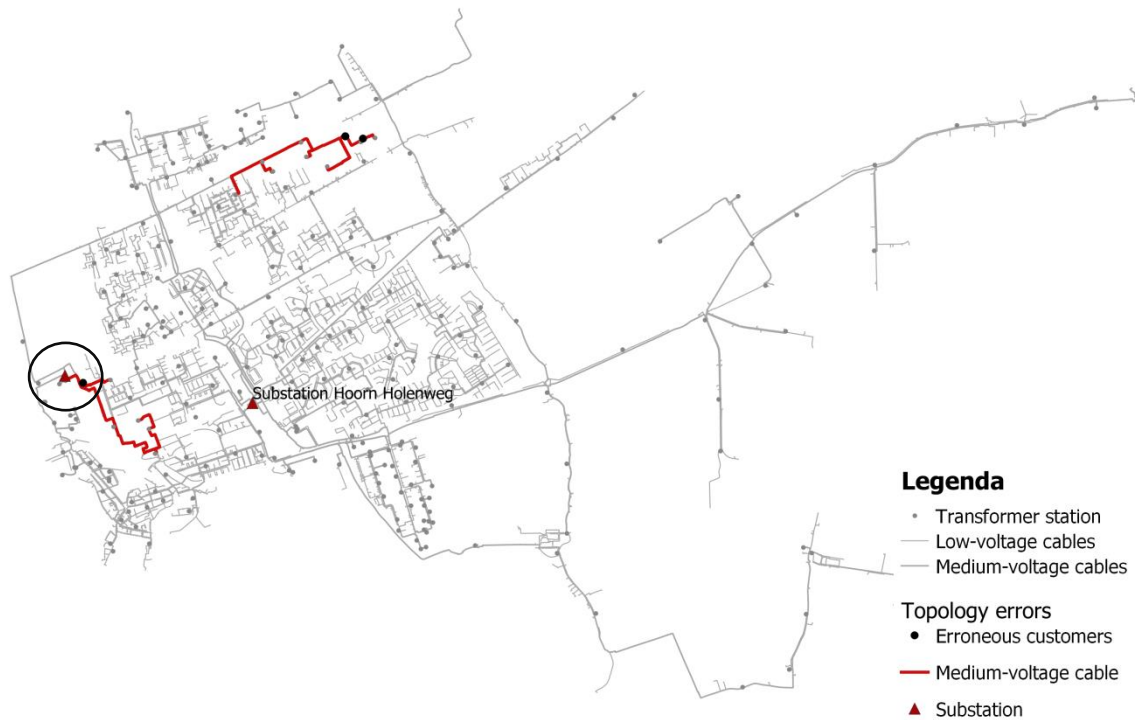
Figure 1: Erroneous medium-voltage distribution network.
