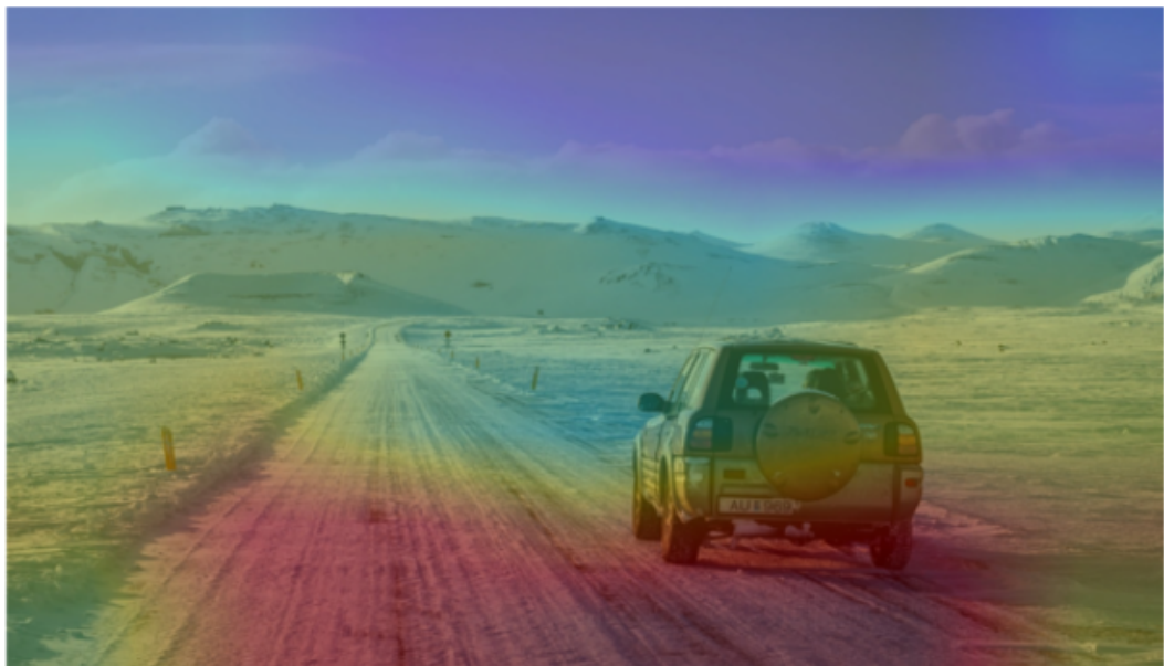
Fig. 5.6: An image of rural Iceland with snow on the driving surface. We overlaid the class attention for the class snow on a blue to red color ramp. Red colors indicate a higher class attention. The model's confidence for the class snow in this image is 99.5%. Notice how despite that the image contains snow everywhere, the only snow in focus is on the surface itself. Original image source: [47]
