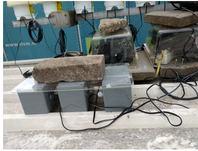
Figure 3.10: Set up of the calibration system of the static sensors. The three static sensors are placed next to each other, all with the sensor side turned inwards. On top of it a plastic screen is placed with a brick on top to keep the plastic screen on its place.
