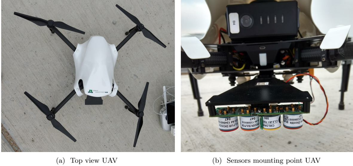
Figure 3.1: Figure 3.1a shows the above view of the UAV used during this research. It is the UAV DJI Matric 100, owned by RIKILT Wageningen University and Research. Figure 3.1b shows how the sensors are mounted underneath the UAV. The sensors are the AlphaSense sensors for \text{NO}_2 , \text{CL}_2 , \text{H}_2\text{S} and \text{SO}_2 , all of the A42F series, the series which are specially designed to be smaller and useful for mobile platforms.
