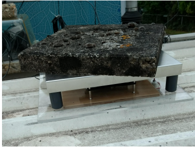
Figure 3.9: Set up of the UAV sensor for outside calibration. The sensors are attached to the plastic at the bottom. On top of it an aluminum screen is placed which protects the sensor from rain. The rock is placed on top to keep the aluminum screen on its place. Still enough space was opened at all sides to get enough airflow through.
