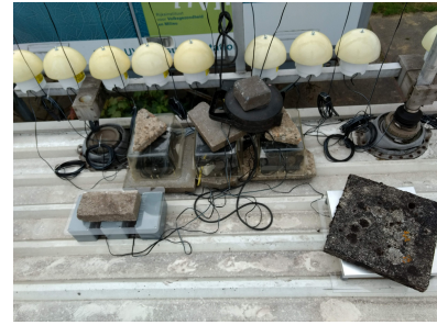
Figure 3.11: The complete set-up of the outside calibration system with the UAV sensors at the complete right, static sensors at the complete left and the RIVM official sensors in the white mushrooms on the background.
