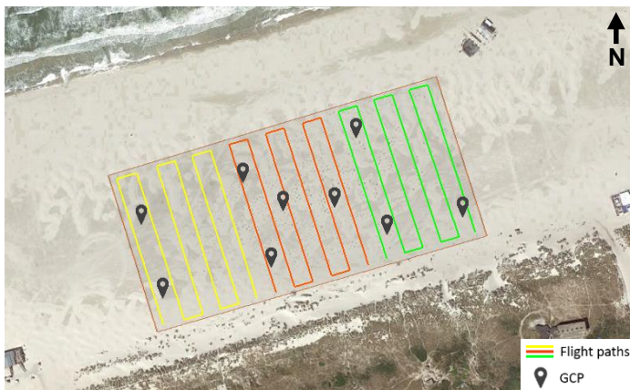
Figure 6 Flight paths for data collection visualized with GCP locations
