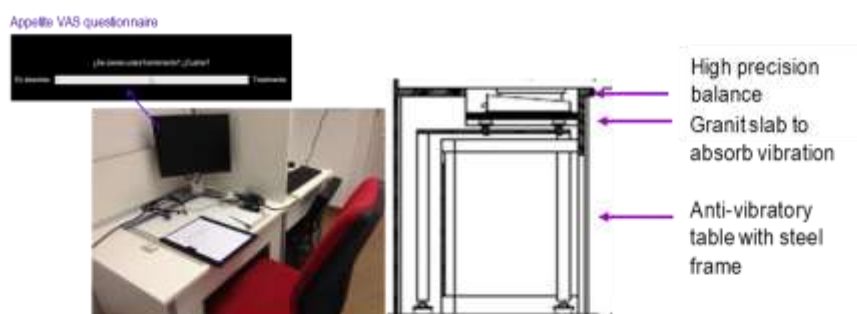
Figure 4. Universal Eating Monitor station at the University of Navarra. Diagram courtesy of Borda Laboratorios, Madrid, Spain.
