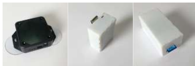
Figure 2: modules to locate multiple persons: anchor (left), tag (middle), mastertag (right)
