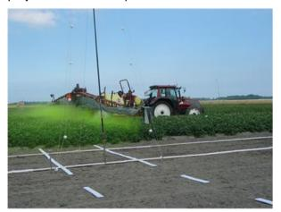
Figure 1: Tractor and Hardi Commander sprayer driving through potato field, parallel to a bare soil field. Filter strips parallel to the field edge allow measuring variation in spray drift deposits along the edge.
