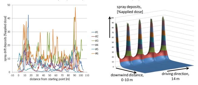
Figure 2: Left: measured spray drift deposits at 2 m downwind from the treated field, as a function of distance alongside the field; 6 repetitions are shown; right: simulated spray deposits downwind for sinusoidal horizontal sprayer boom movements at 0.50 Hz
