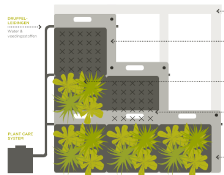
Figure 8 | Schematic drawing of pre-grown panels by Sempergreen (Sempergreen, 2018)
