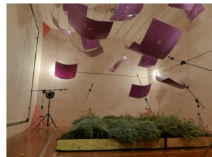
Figure 18 | Testing absorption coefficient in a reverberation room (Azkorra et al., 2015, p.
