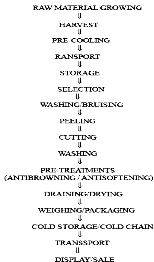
Figure 6 - Flow-sheet of fresh-cut horticultural products processing
