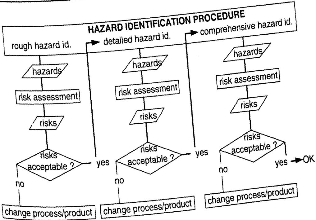
Fig. 2. Process of using several levels of detail in the hazard identification procedure (Van Gerwen et al., 1997).
