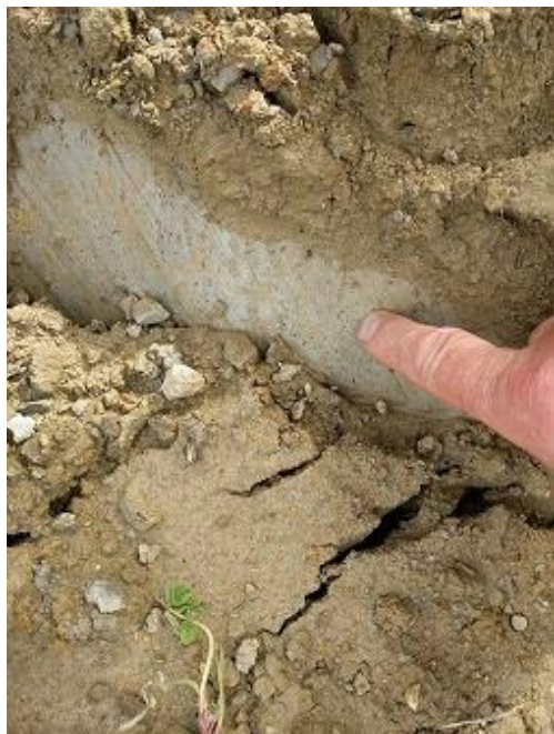
Figure 3.8. Smeared surface on landslide shear plane (23-03-2016, Collazzone study area in Italy).
