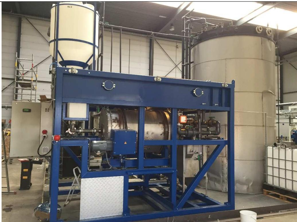
**Figure 4.4 Pilotplant Elemetal / Inashco for recovery of copper and other metals from non-ferrous fractions**
