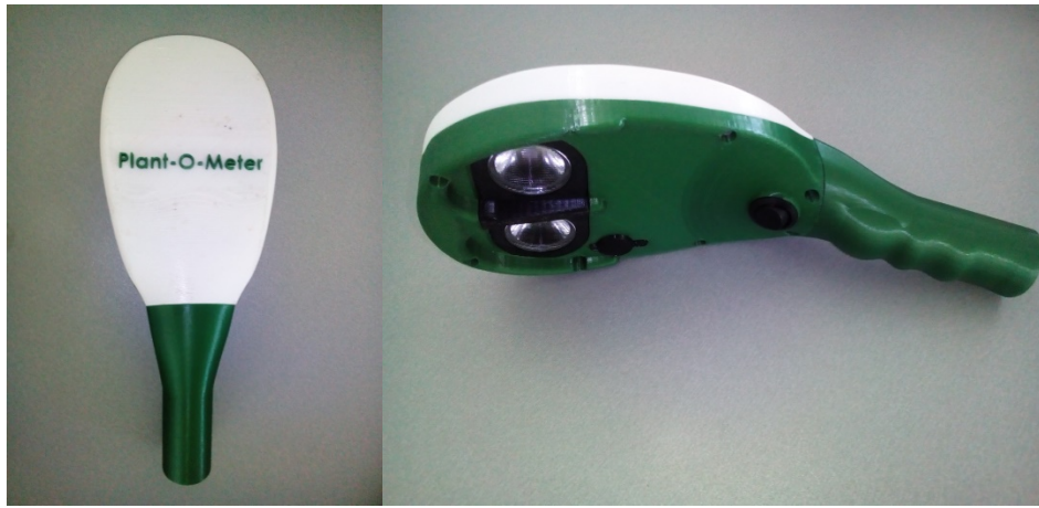
Figure 4. Plant-O-Meter active proximal crop sensor developed by BioSense.
