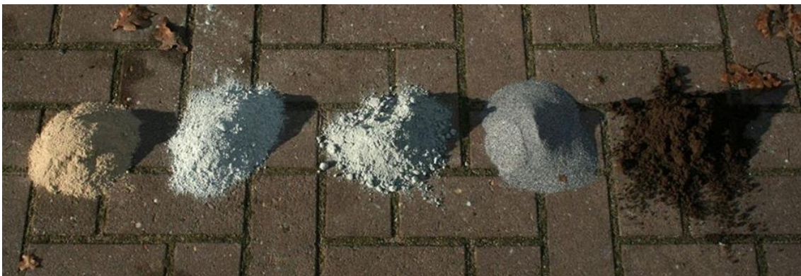
Photo S.1. Various buffer agents used in the experiment in Strabrecht. From left to right: Dolokal, Biolit (fine grind), Biolit (coarser grind), Lurgi and Lavagruis.
