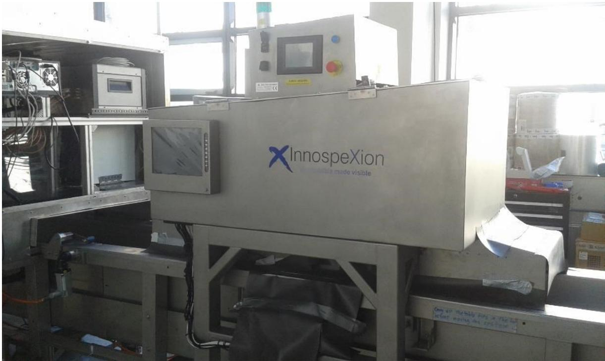
Figure 1. The X-ray sub-module in the PicknPack Line.
