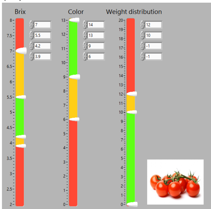
Figure 23. Screenshot of (a part of) the user interface to define quality classes for tomato trusses. The colours on the sliders indicate the desired values for each feature (green: premium quality, orange, acceptable, red: not acceptable).
