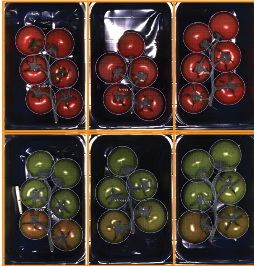
Figure 10: Examples of segmentation of the raw image data to the separate packages (orange boxes), identification of the individual tomatoes (blue ellipses), and stalk/calyx (blue dotted regions).
