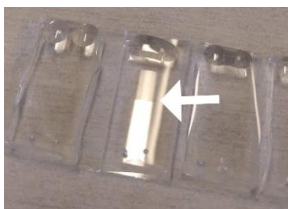
Figure 56 Epoxy resin is added on top of the PDMS structure. The epoxy resin fills the mould through the punctured holes via capillary action. The arrow indicates the epoxy interface; the mould is filled half-way in this picture. Filling takes ~20 minutes.
