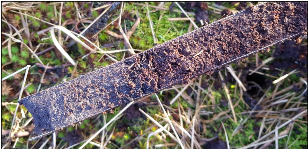
FIGURE 5.4: PHOTO OF THE SHARP TRANSITION BETWEEN THE PEAT AND THE COVER SAND AT CP29B.
