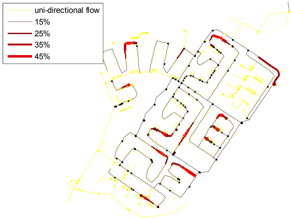
Figure 8-8. Percentage of time that flow direction reverses. 50% means that 50% of the time flow is in one direction, and 50% of the time in the other direction pipes (0.01 h time step).
