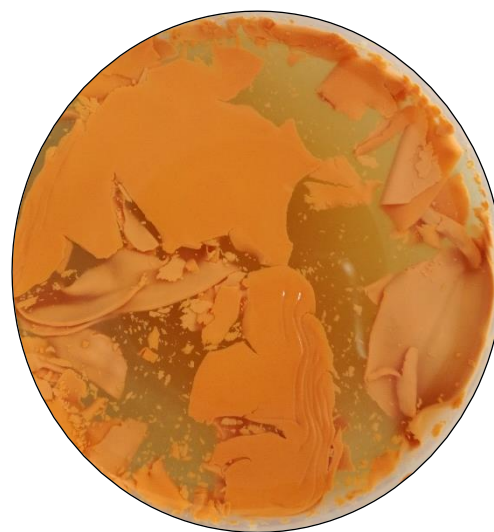
Figure 4-6. The equivalent of OBC-1 obtained from aqueous extraction of pomace at pH 9. Flakes were unstable and dissolved quickly in the underlying subnatants.
