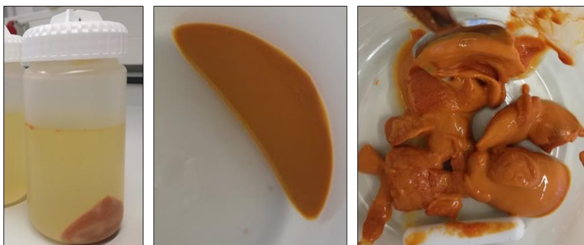
Figure 4-7. The red pellet produced by enzyme-assisted aqueous extraction of tomato pomace. Left: centrifugation bottle directly after centrifugation. The yellowish supernatant was discarded. Middle: Pellet from above, without supernatant. Right: pellet once scooped out of the centrifugation bottles.
