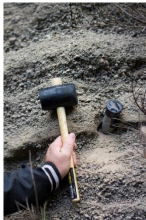
Figure 8: Tube inserted in scoria wall for OSL sampling. Hammer for scale
