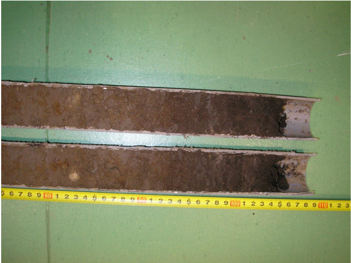
Figure A4: Photograph the BP5 core that was used for DR measurements. It shows the boundaries between the fAh (>102cm), the transition of fAh to colluvium (M-fAh) (90-102cm) and the colluvium (M) (<90cm), that do not show clear parabolic shapes that would be signs of strong influence of friction at the core wall during sampling.
