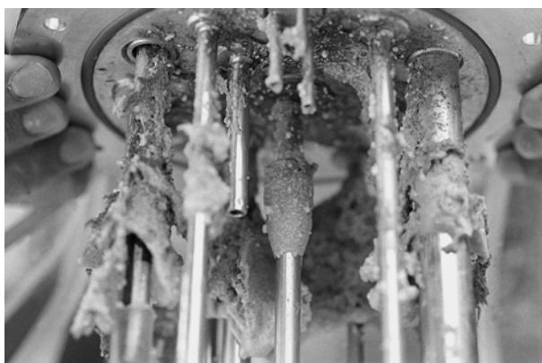
Figure 2. Massive accretion of A. oryzae biomass on headspace surfaces in a conventional Applikon BTS 0.5 bioreactor. A. oryzae was grown in batch culture on minimal medium with glucose as final cell density limiting substrate. After glucose exhaustion, the bioreactor was autoclaved and the head-plate removed.
