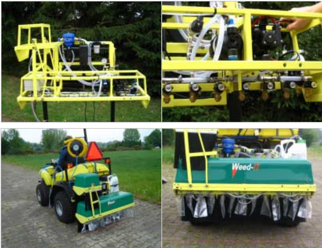
Figure 4. Sprayer hardware of the Weed IT 2006 MKII, with a nozzle sensor unit every 8 cm. On bottom row, pictures of spray release sampling with plastic bags over each nozzles.
