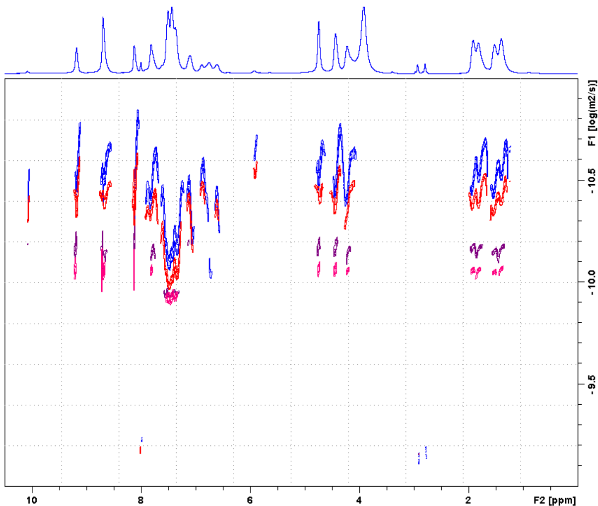
Figure 23: Overlaid DOSY spectra of compound 8 in a 20% w/v solution of DMF-d 7 (pink), and with an addition of 0.1 (purple), 0.2 (red) and 0.3 (blue) equivalents of Eu(III)(OTf) 3 . With the chemical shift on the x-axis and the 10Log of the diffusion coefficient on the y-axis. The signals with a ppm between 2.5 and 3.5, and the one at 8 originate from the solvent (DMF-d 7 ), those between 6 and 7 belong to free aniline.
