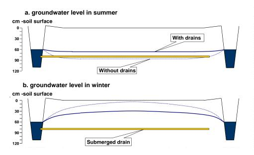
Fig. 1: Reduction of peat oxidation and subsidence and CO<sub>2</sub>-emissions by raising groundwater levels with infiltration via submerged drains in summer level. In wet periods the submerged drains will function as drainage.
