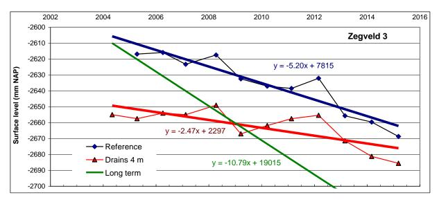
Fig. 2: Subsidence 2004 – 2015 of peat soil without submerged drains (Reference) and with submerged drains at a distance of 4 meters (Drains 4 m). The long term subsidence is 10.8 mm per year. NAP = the Dutch national reference level, which is about the average sea water level.
