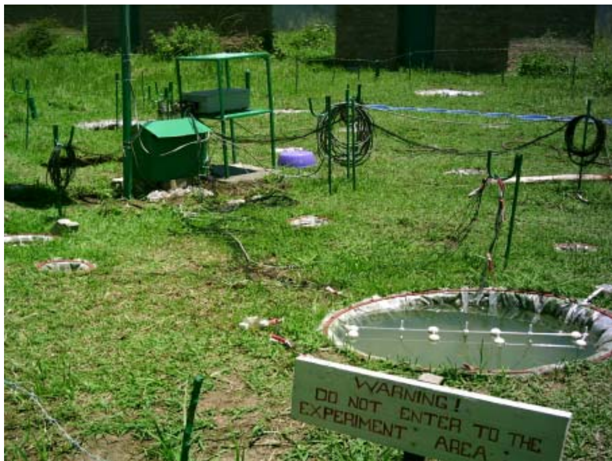
Figure 1.5 Automated micrometeorological stations at KEMRI, measuring water temperatures in various semi-natural water bodies and soil temperatures at various depths.
