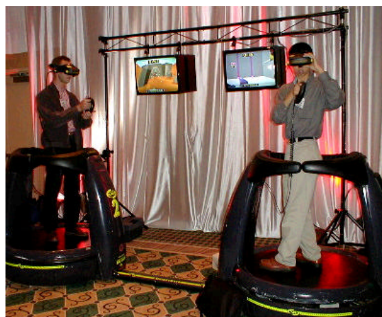
Figure 5: An example of the hardware environment (pods) visible to a player. Each player wears a see through head-mounted display and interacts with a personal interaction panel.
