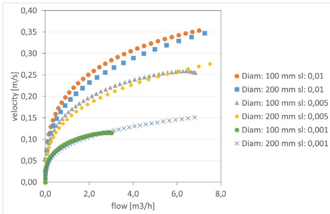
**Figure 21 Relation between velocity, flow, diameter and slope for partially filled pipes. The flow is relevant for maximum domestic water use (and waste water production) for 20-40 houses (Vreeburg, 2017).**
