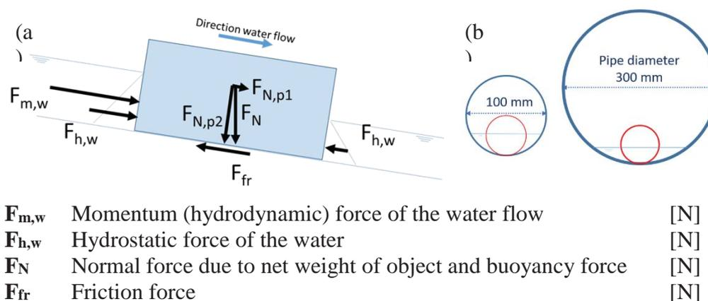
**Figure 22 (a) Forces on an object in a sloped pipe (Vreeburg, 2017); (b) With the same amount of flow, the water depth behind the object in a smaller diameter sloped pipe is higher and offers more buoyance for transporting the object.**
