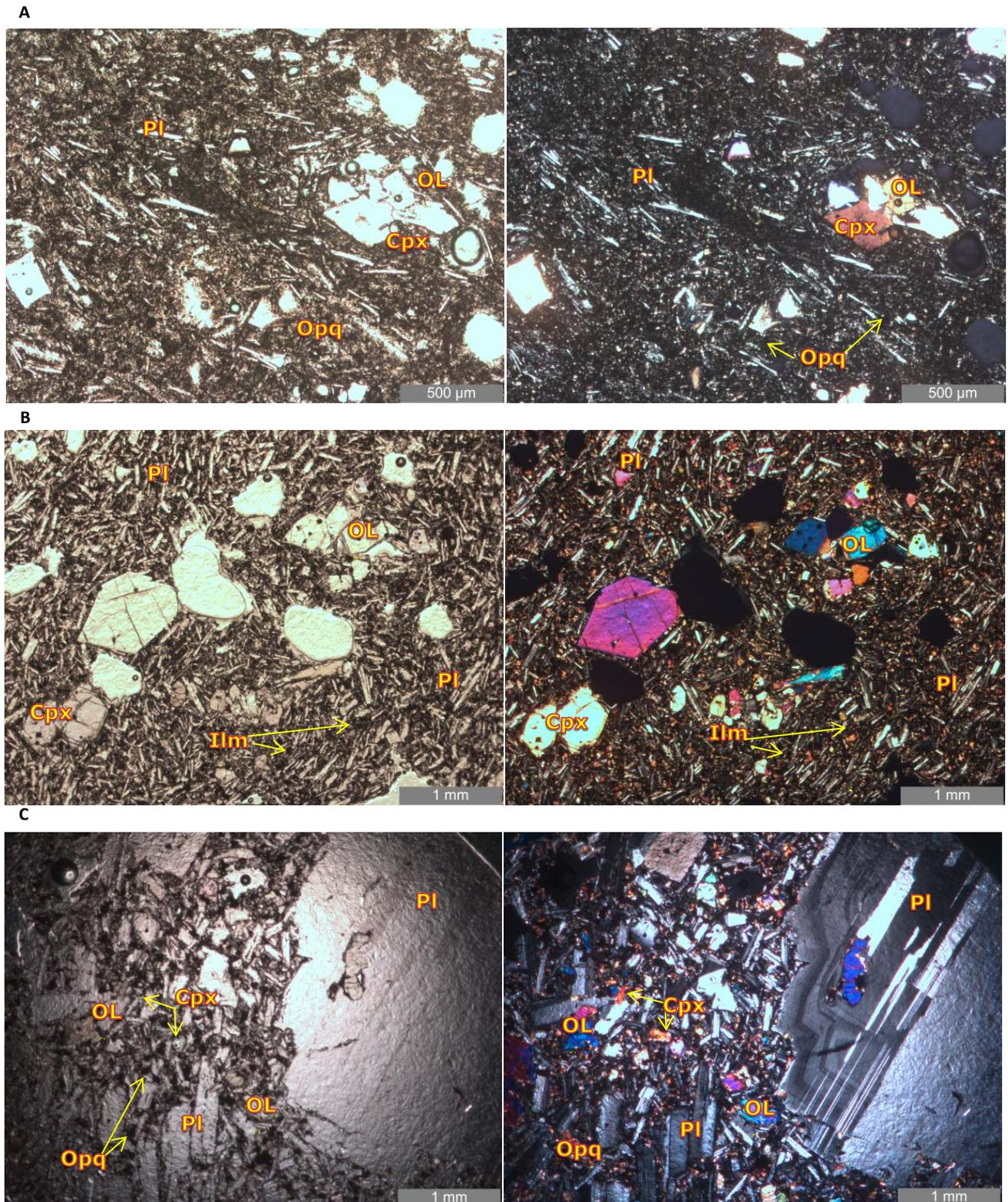
Figure 2.4.1 Examples of images from the Leica Polarising microscope. Left: Plain polarised light, right: crossed polarised light. A) PI-08 lacking significant phenocryst phases, with abundant magnetic minerals. B) PI-04 with only olivine and pyroxene phenocrysts and a coarse feldspar-rich groundmass. C) PI-19 with large plagioclase phenocrysts and a coarse groundmass (>0.5mm). Pl: plagioclase, Ol: olivine, Opq: opaque minerals, Ilm: Ilmenite, Cpx: clinopyroxene.
