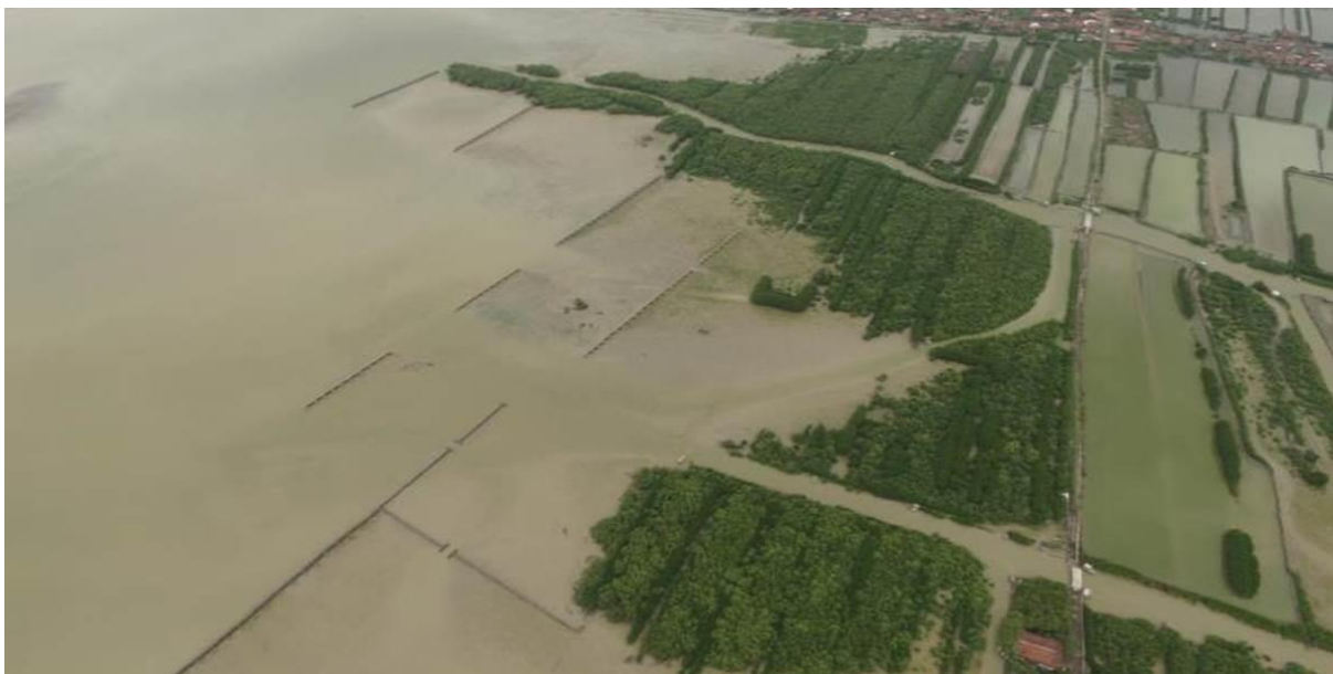
Figure 4. Aerial view of permeable dams at the pilot project location
