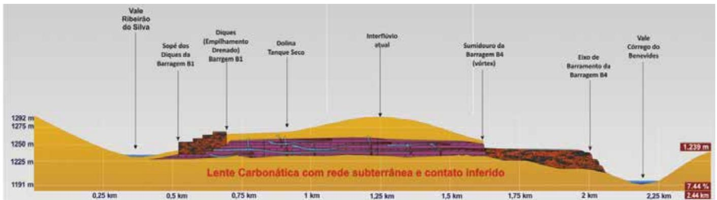
Fig. 64: Schematic section of the channel system under the Herculano's Plateau. Source: BRANDT 2015
