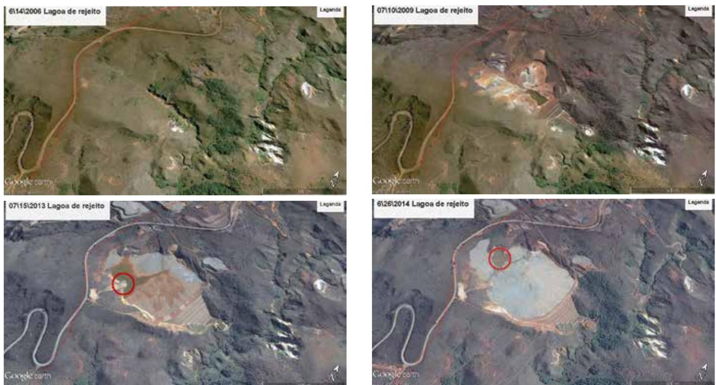
Fig. 65: Chronology of the tailings dam B4: 2006) when the dam was not yet constructed, 2009) when the construction started, 2013) when almost at its maximum height the water started moving from the overflow towards the karstic formation and 2014) when the water had entirely moved upstream. Source: Internet
