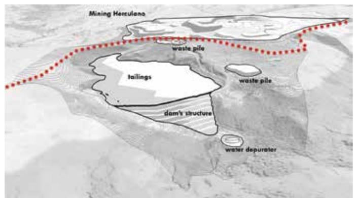
Fig. 19: Partition of the tailings dam B4. Source: Original image
