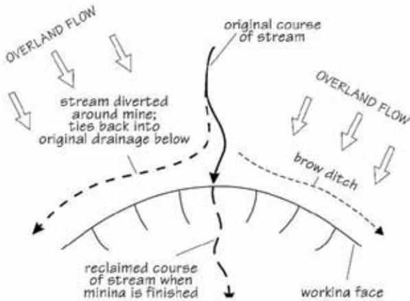
Fig. 115: Storm water diversion scheme. Source: Norman (1997)
