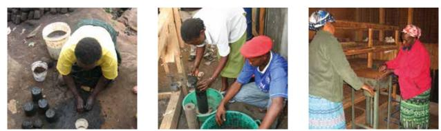
(a)Charcoal briquettes moulding in recycled plastic containers and (b) compacted in wooden manual press and (c) sawdust briquettes compacted using metal manual press. All photos by Mary Njenga
