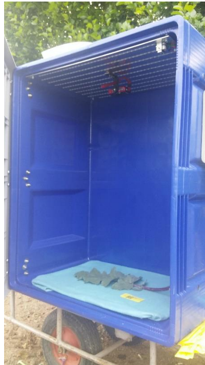
Figure 3.2.1 Picture to illustrate the use of the photo box. At the top of the box ten LEDs and a camera are installed. At the bottom a leaf with a corresponding label are placed on a light blue cloth.
