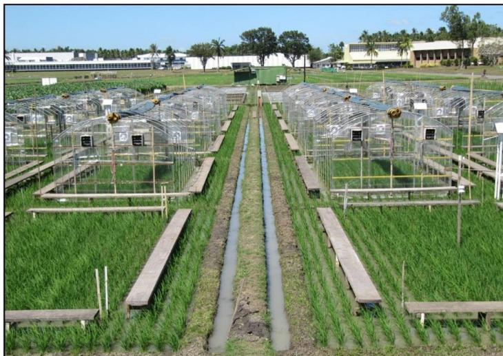
**Figure A2.1** Field growth chambers used to study high night-time temperature responses
