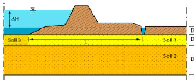
Figure 2: Schematization of the piping mechanism for the Floris-2 project
