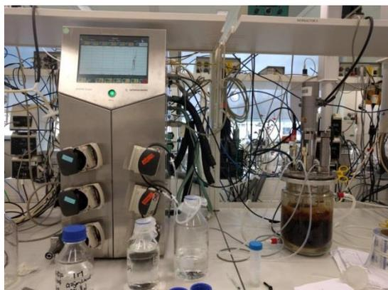
Figure 7. Reactor set-up for the PHB accumulation experiment in TU-Delft.
