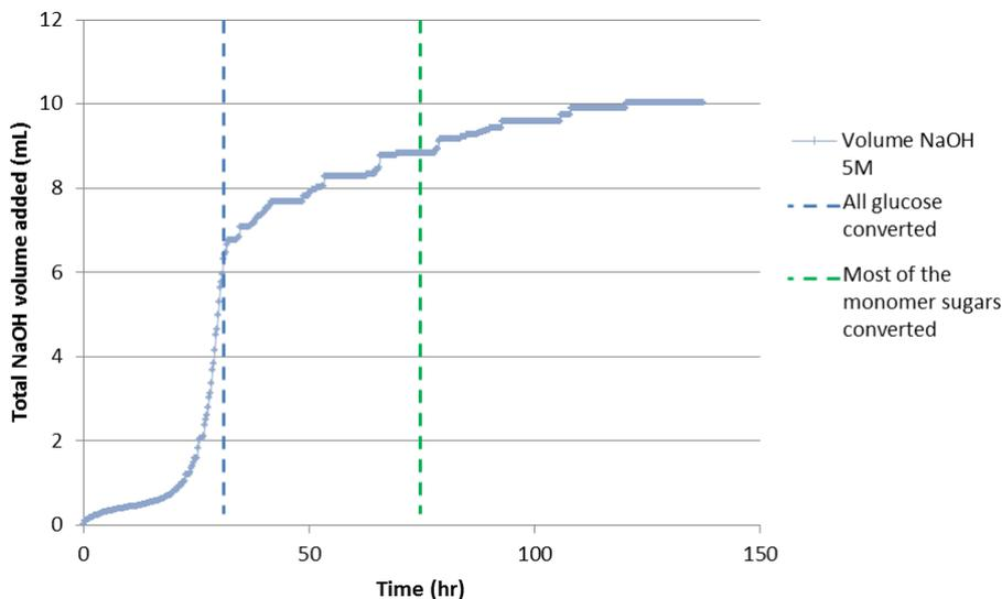
Figure 18. Sodium hydroxide addition during the acidogenic fermentation. Starting concentration pyrolytic sugar was 10% (v/v).
