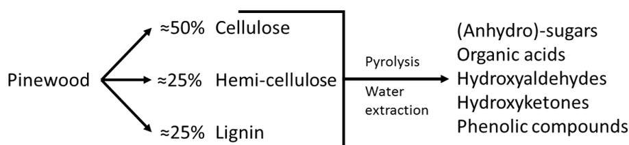
Figure 2. Overview of the organic composition change during the pyrolysis and water extraction.
