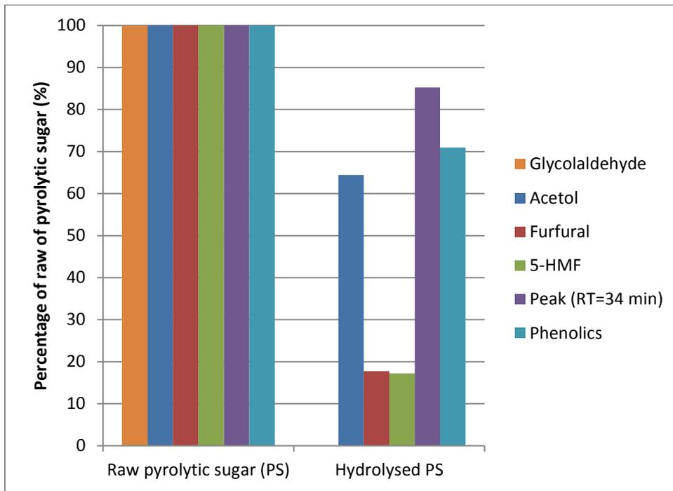
Figure 11. Inhibitory removal comparison between raw pyrolytic sugar and the hydrolysed sample. Hydrolysis time was 60 minutes at 120 °C
