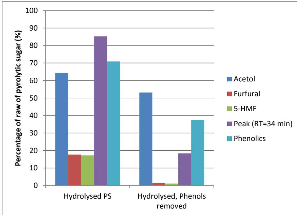
Figure 12. Inhibitory removal comparison between hydrolysed pyrolytic sugar and hydrolysed and XAD-4 treated pyrolytic sugar. Resin retention time was 20 hours at 25 °C
