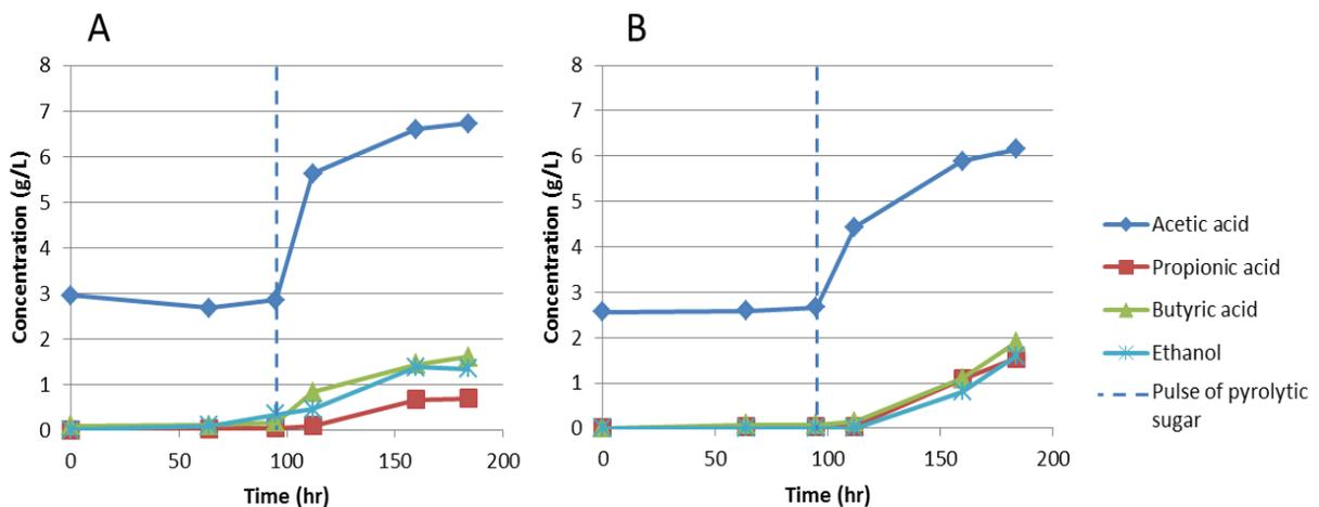
Figure 20. Product concentration profiles during the acidogenic fermentation. On the Left (A), fermentation with nitrogen limited conditions (100 mg NH<sub>4</sub>/L). On the Right (B), control fermentation with carbon limitation (500 mg NH<sub>4</sub>/L). Starting concentration was 10% (v/v) pyrolytic sugar.
