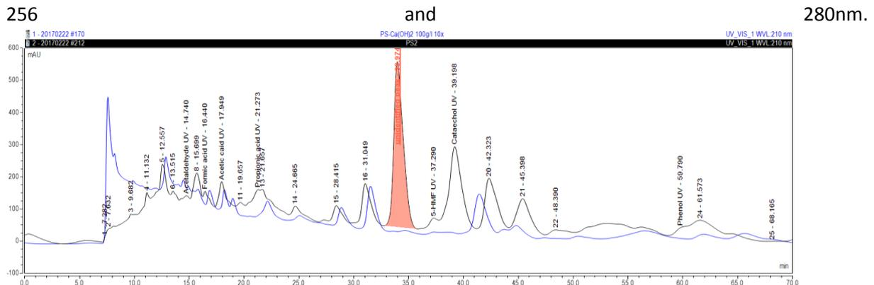
Figure 9. HPLC chromatogram comparison between raw pyrolytic sugar (black) and calcium overlimed pyrolytic sugar (blue). Detection is at 210 nm with a run time of 70 minutes.
