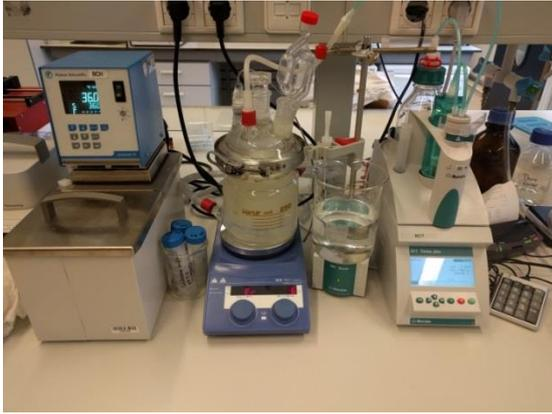
Figure 5. Set-up for the acidogenic fermentation
