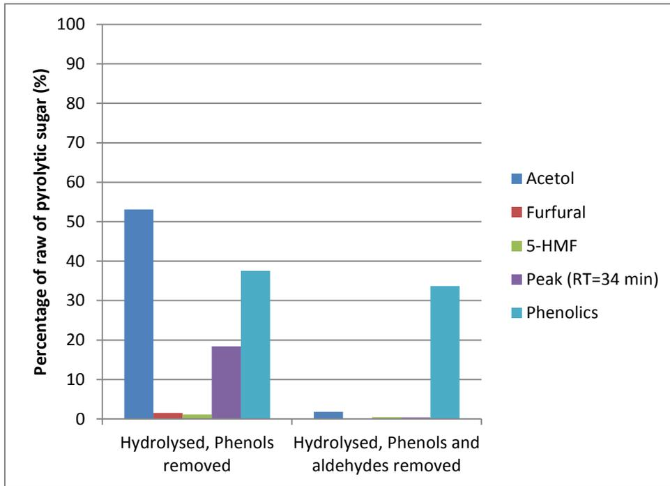
Figure 13. Inhibitory removal comparison between hydrolysed and XAD-4 treated pyrolytic sugar and hydrolysed, resin treated and vacuum evaporated pyrolytic sugar. Water bath temperature was 80 °C and pressure was reduced to 40mbar for 1 hour.
