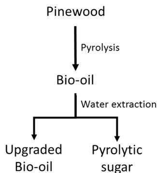
Figure 1. Schematic overview of obtaining pyrolytic sugar.
