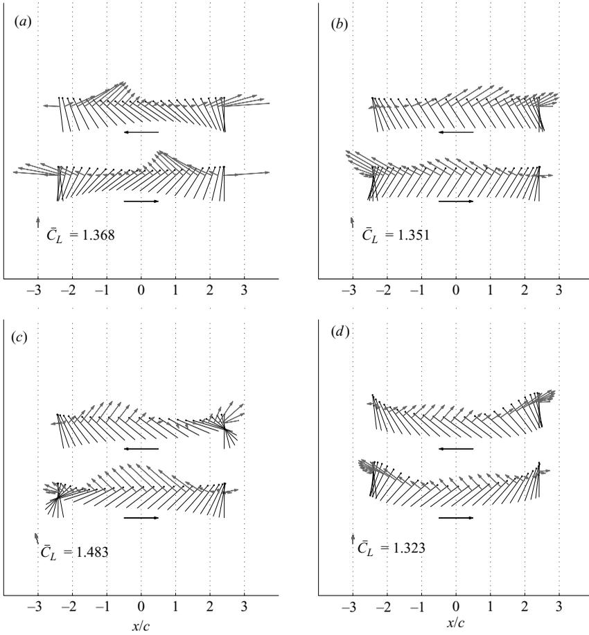
FIGURE 12. Force vectors during each half-stroke. (a) harmonic model with sawtooth  $\phi$ , (b) harmonic model with trapezoidal  $\alpha$ , (c) harmonic model with extra bump  $\alpha$ , (d) harmonic model with deviation  $\theta$ .
