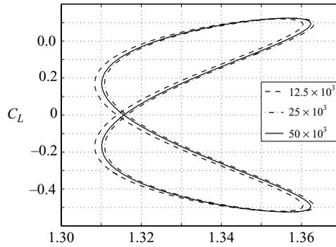
FIGURE 25. Phase Diagrams of unsteady flow around a static cylinder at  $Re = 150$  and the corresponding limit cycles. The knot at  $C_L = 0$  shifts to the left according to  $25 \times 10^3$ ,  $50 \times 10^3$  and  $12.5 \times 10^3$  cells.
