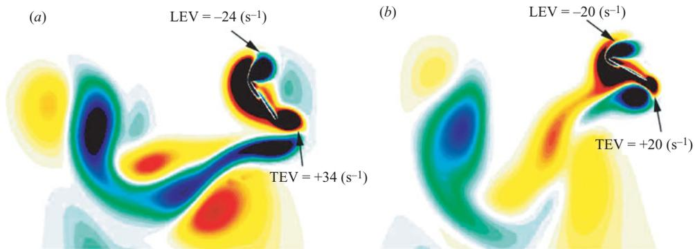
FIGURE 11. Vorticity contours at  $t = 0.1T$  (blue: clockwise, corresponding to negative vorticity values) (a) harmonic model, (b) realistic fruit fly model. LEV denotes leading-edge vortex and TEV trailing-edge vortex.
