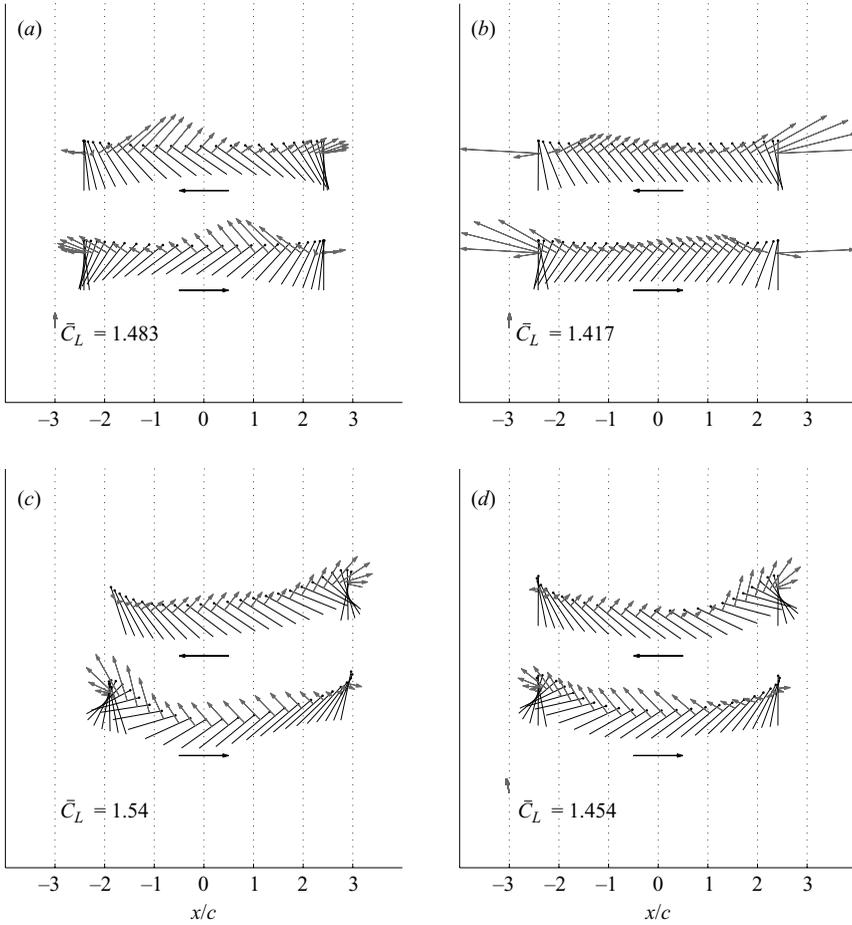
FIGURE 10. Force vectors during each half-stroke. (a) harmonic model, (b) RoboBfly model, (c) realistic fruit fly model, (d) symmetric fruit fly model.
