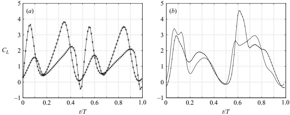
FIGURE 8. Lift force histories of the baseline kinematic models: +, harmonic model; ×, Robofly model; ●, realistic fruit fly model; —, simplified fruit fly model.
