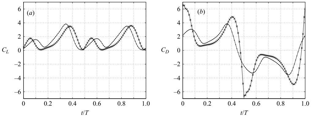
FIGURE 13. Force histories to investigate the influence of the sawtooth displacement compared to the harmonic model:  $\bullet$ , harmonic  $\phi, \alpha, \theta$ ;  $\times$ , harmonic  $\alpha, \theta$  and Robofly  $\phi$ .
