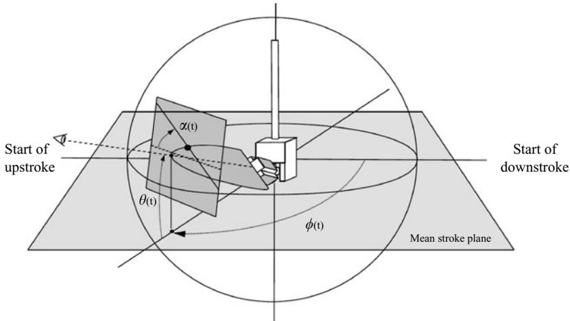
FIGURE 5. Illustration of the main motion directions.  $\phi(t)$  corresponds to the stroke variation,  $\alpha(t)$  to the geometrical angle of attack and  $\theta(t)$  to the deviation from the horizontal stroke plane. Source: Sane & Dickinson (2001). Reproduced with permission of the Company of Biologists.
