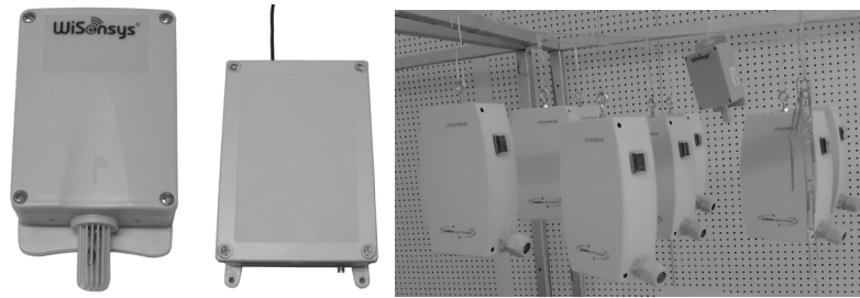
Fig. 2. Wisensys node (left) and the base station (middle). Wisensys node accuracy test in comparison with other sensor nodes in a climate chamber (right).
