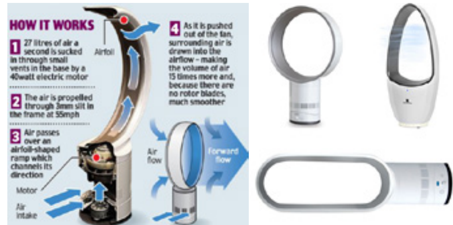
Illustration 92: Mechanism of bladeless fans ( www.dailymail.co.uk )
