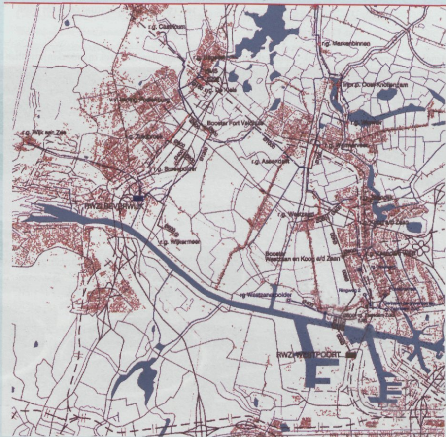
Fig. 1: Area layout for the alternative Westpoort. In this case wastewater has to be pumped from Assendelft to sewage plant Westpoort instead of sewage plant Beverwijk.
