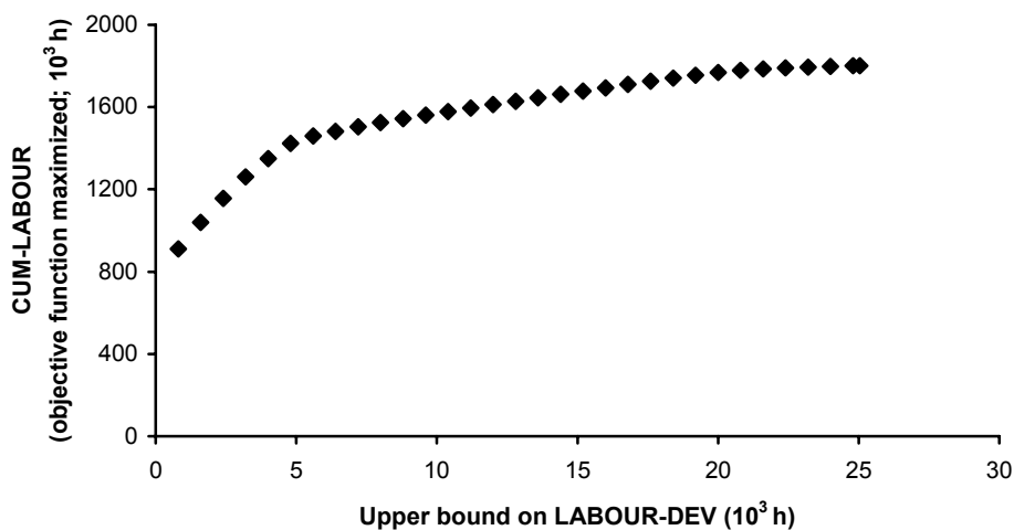
Fig. 5. Trade-off between CUM-LABOUR (objective function that is maximized; 10^3 h) and upper bound on LABOUR-DEV ( 10^3 h) during the November-April period.
