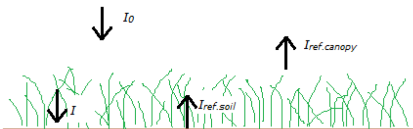
Figure 3.2. Overview of the four radiation fluxes that have been measured to obtain the absorbed PAR by the canopy.
