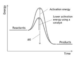
Figure 10: Principle of catalysis
