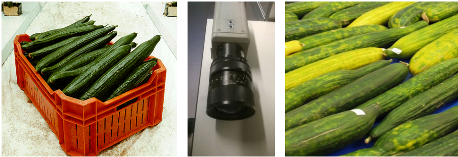
Figure 5. Based on colour measurement at harvest a model can predict shelf life of cucumber fruits. From Schouten et al. (2002; 2004).
